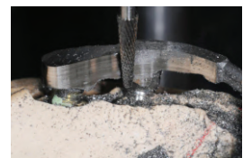
Bar Milling after Casting
